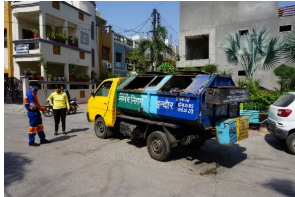
Collection vehicles with separate chambers for different waste materials
